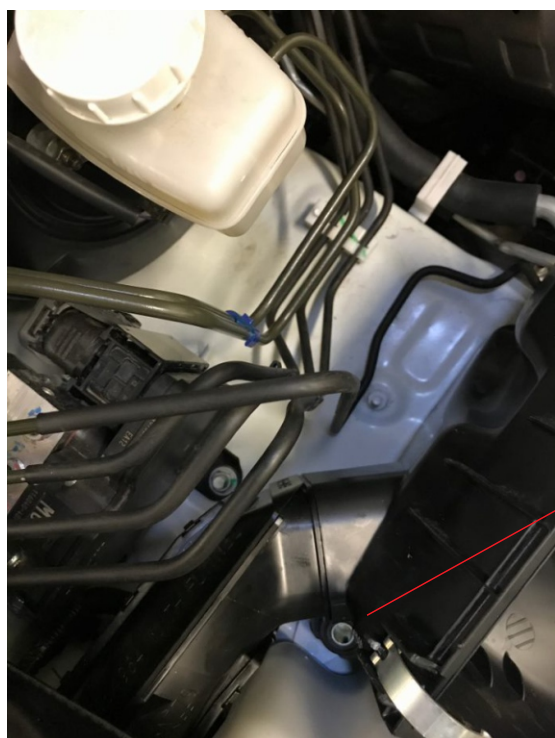
FIG. 8b AIRBOX MOUNTING OEM BOLT/WASHER REMOVAL
